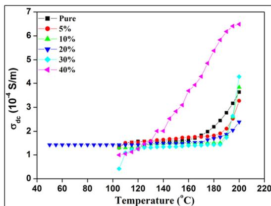
Fig. 4. DC Conductivity of Pure Polyaniline and doped Ag<sub>2</sub>O (5%, 10%, 20%, 30%, 40%).
