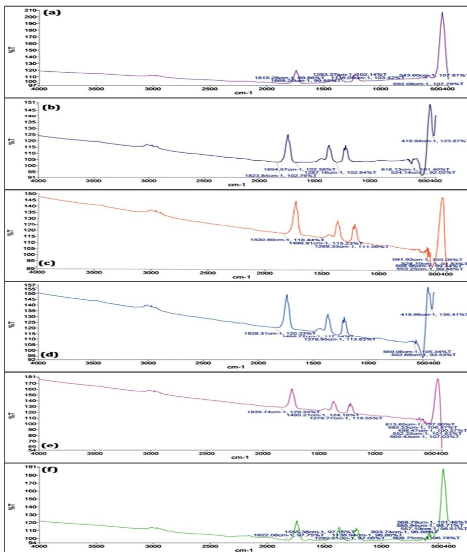
Fig. 3. FTIR spectroscopy of Pure Polyaniline and doped Ag<sub>2</sub>O (5wt%, 10wt%, 20wt%, 30wt%, 40wt%).
